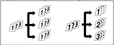
Prints two pages of originals on both front and back sides of a single sheet of paper.
